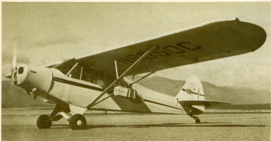
The PA-18 "Super Cub" was a higher-powered development of the PA-11. Principal recognition feature from a distance was the more rounded rudder adapted from the three-seat J-5C and PA-12. This PA-18-135 carries salt blocks on wing bomb racks for airdrop to livestock in the western mountains.
