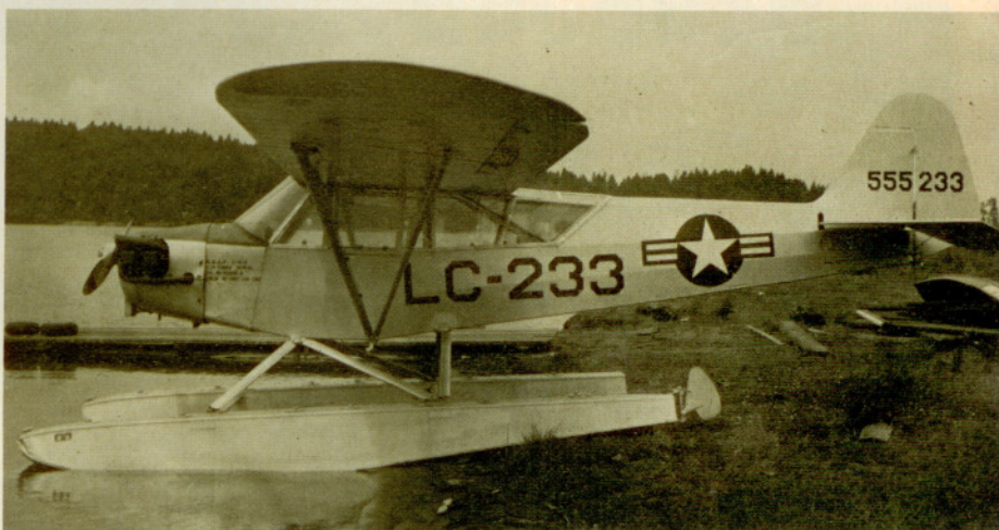
Army J-3 was originally called O-59 but was redesignated L-4 in 1942. L-4A and subsequent models had transparent section behind the wing. This is rare seaplane version of L-4J. L-18 and L-21 were similar military versions of 90 hp and 125 hp PA-18 "Super Cubs." Photo by Peter M. Bowers
